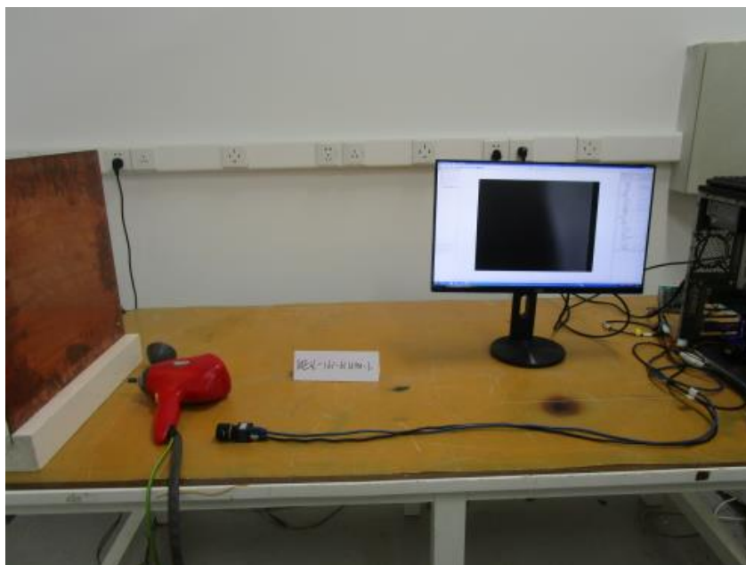
Photograph 2: Set-up for immunity test of electrostatic discharge
