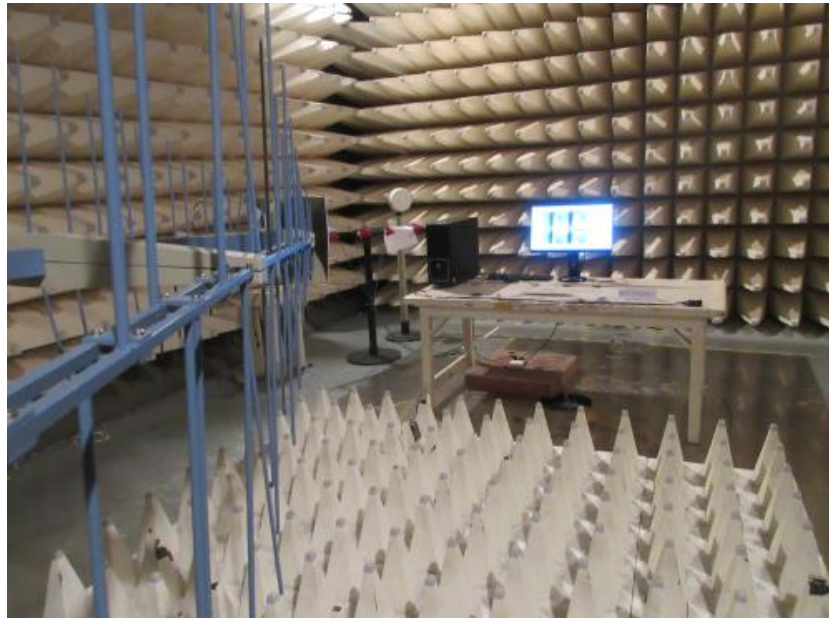
Photograph 3: Set-up for immunity test of RF electromagnetic field
